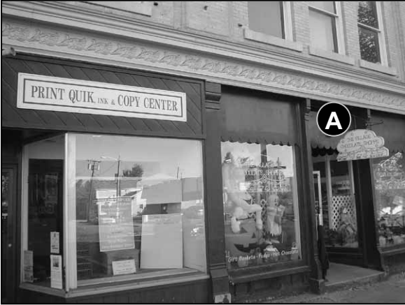
Fig. 5-88: 471 Main St. Hanging signs like this often are the least obtrusive to the architecture of the original façade.
